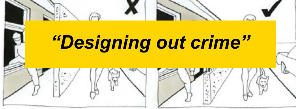
Figure 7. Solid fencing prevents visibility but permeable or semi-permeable fencing promotes natural surveillance
